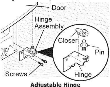
To reinstall the refrigerator door, reverse the above steps.
