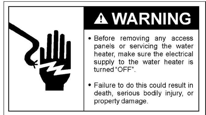
1. Before beginning, turn "OFF" the electric power supply to the water heater. After the power has been turned off, open a nearby hot water faucet until the water is no longer hot.
