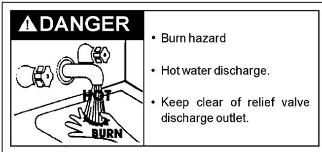
The temperature-pressure relief valve must be manually operated at least once a year. Caution should be taken to ensure that (1) no one is in front of or around the outlet of the temperature-pressure relief valve discharge line, and (2) the water manually discharged will not cause any property damage or bodily injury. The water may be extremely hot.
