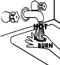
Water temperature over 125°F (52°C) can cause severe burns instantly resulting in severe injury or death.
