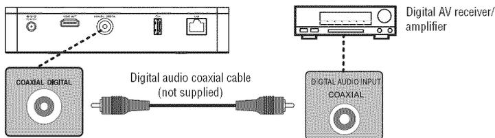
(Sample Illustration) Connecting to a digital AV receiver/amplifier
