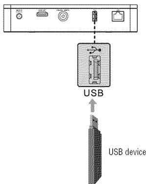
(Sample Illustration) Connecting a USB device
