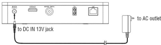
(Sample Illustration) Using AC adapter
