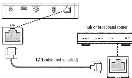
(Sample Illustration) Connecting to a wired router
