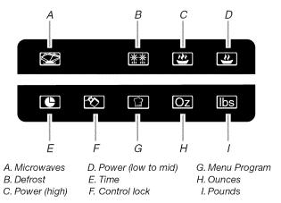
The icons light up in the display while their specific functions are being programmed. While the set function is operating, the icons flash until the program is over. The control lock icon remains lit – not flashing – while the control is locked.
