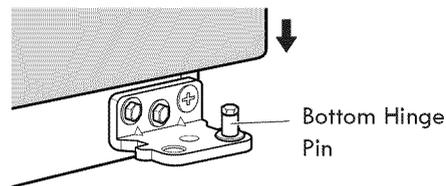
8. Using a 1/4 in. socket wrench, loosen and remove the hinge pin from the bottom hinge.
