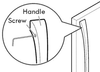
2. Loosen the handle mounting fasteners with a 1/4 in. Allen wrench.
