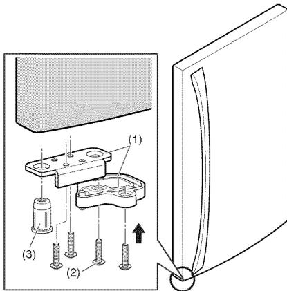
6. Use a 1/4 inch hex socket wrench to loosen and remove the hinge pin (1) from the middle hinge bracket. Use a 10mm or 13/32 in. socket wrench to remove the two bolts (2). Remove the screw (3) and set the middle hinge bracket (4) and other parts aside.
