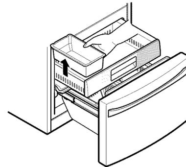
**⚠ CAUTION:** Pinch hazard! Keep hands and feet clear of the bottom of the freezer drawer when opening and closing.
