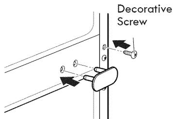
12. Loosen the two screws and remove the left hinge cap.
