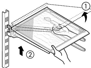
**To reinstall a shelf** — Tilt the front of the shelf up and guide the shelf hooks into the slots at a desired height. Then, lower the front of the shelf so that the hooks drop into the slots.
