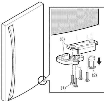
5. Reinstall the hinge pin brackets (1), screws (2) and hinge pin insert (3) on the bottom left side of the door.
