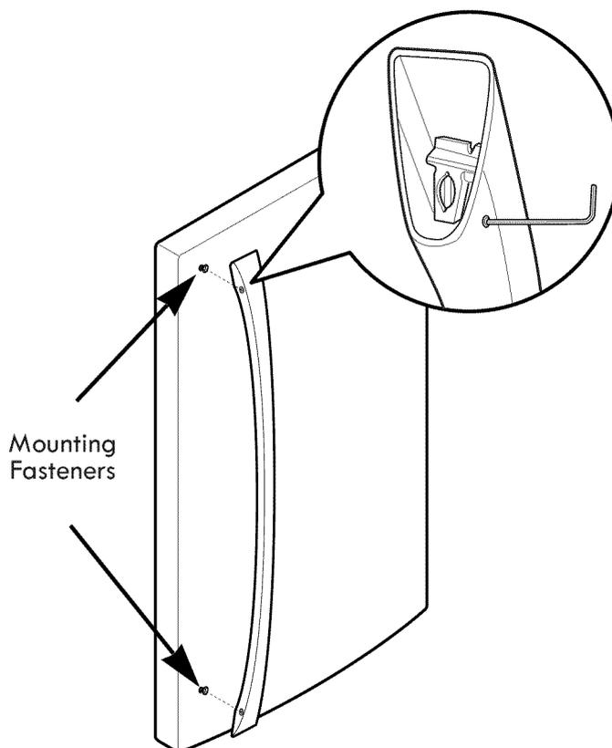
**NOTE:** Removing the doors is the recommended procedure when it is necessary to move the refrigerator through a narrow opening. If it is necessary to remove the handles, follow the directions below.
