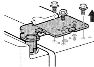
⚠ **CAUTION:** When removing the bolts, be careful that the door does not fall forward.
