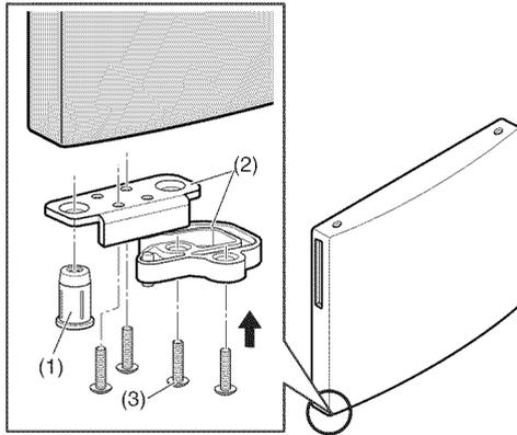
12. On the top part of the door, you will find a cap (1) and a pivot (2). Remove it with a flat head screwdriver and install it on the opposite side ( the cap stays on the right and the pivot on the left).
