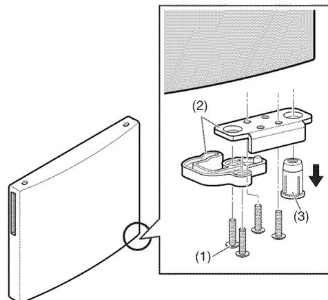
11. Reinstall the hinge pin insert (1), the hinge pin brackets (2) and screws (3) on the bottom left side of the door.
