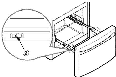
Grasp the drawer on each side and pull it up to separate it from the rails.
