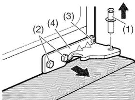
7. Carefully lift up the freezer door. Remove and place it on a non-scratching surface.
