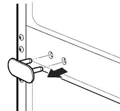
8. Remove the outer lower decorative screw from the flange on the frame between the freezer and refrigerator doors. (You will need this hole for the middle hinge bracket.)
