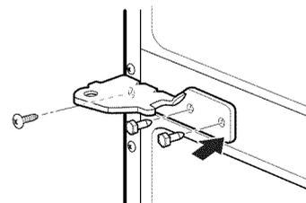
10. Reattach middle hinge pin using 1/4 in. socket wrench.
