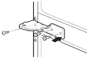
19. Place freezer door down on bottom hinge pin.
