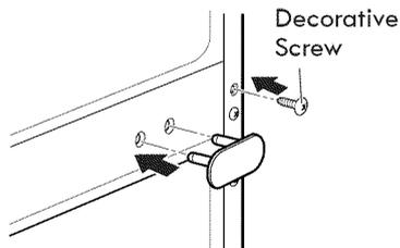
22. Loosen the two screws and remove the left hinge cap.
