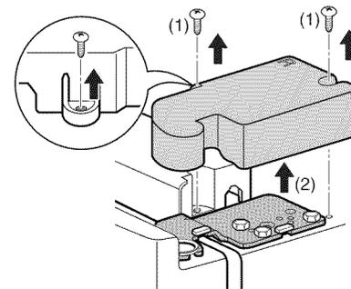
2. Using a 10mm or 13/32-inch socket wrench, remove the three bolts and lift off the top hinge. Set parts aside.
