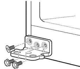
15. Attach the hinge pin using a 1/4 in. socket wrench.
