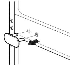
17. Remove the outer lower decorative screw from the flange on the frame between the freezer and refrigerator doors. (You will need this hole for the middle hinge bracket.)
