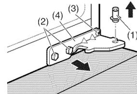
7. With a flat-head screwdriver, carefully pry off and remove the cover over the bolt holes on the left side of the refrigerator.
