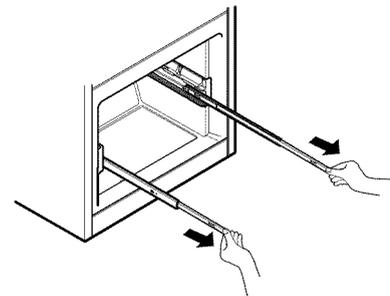
Grasp the drawer on each side and hook the drawer supports ① into the rail tabs ② located on both sides.
