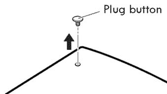
4. Install the plug buttons on the left side.
