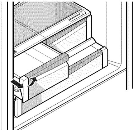
3. To install, slightly tilt up the front, insert the drawer into the frame and push it back into place.
