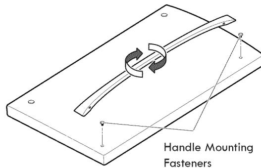
6. Install the handle by adjusting handle footprints to fit the mounting fasteners. Tighten the set screws with a 3/32 in. Allen wrench.
