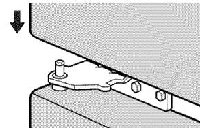
**NOTE:** The left top hinge, left hinge cover and right hinge cap are provided for reversing doors.
