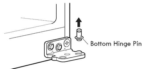
9. Using a 13/32-inch or 10mm socket wrench with a 2 in. extension and a screwdriver, loosen the two bolts and the screw, and remove the bottom hinge on right side.
