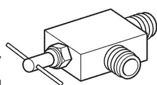
**NOTE:** A Self Piercing Saddle Type Water Valve should not be used.
