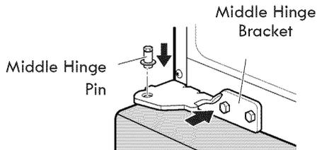
**NOTE:** Bracket has been flipped, but hinge pin stays in the same orientation with its hexagonal end facing upward.
