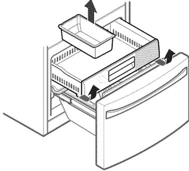
2. To replace, with the drawer pulled out to full extension, insert the top drawer in the rail assembly.
