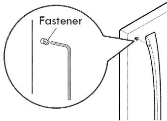
3. Unscrew the buttons with your fingers by rotating counterclockwise; they will loosen and fall free.
