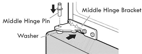
**NOTE:** Bracket has been flipped, but hinge pin stays in the same orientation with its hexagonal end facing upward.
