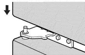
**NOTE:** The left top hinge, left hinge cover and right hinge cap are provided for reversing doors.
