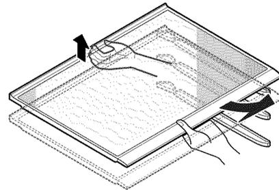
**To reinstall a shelf** — Slide the shelf into the guides until it stops.
