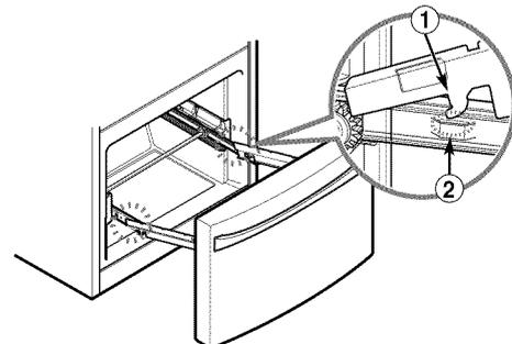
Lower the door into its final position and tighten the screw ③ located on both sides.
