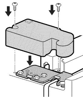
15. Replace the right hinge cap and insert the two screws.
