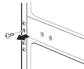
9. Flip the middle hinge bracket and position it on left side of refrigerator. Re-attach with two bolts and a screw.
