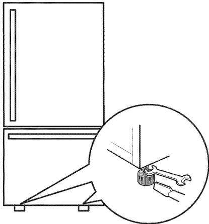
**NOTE:** Having someone push backward against the top of the refrigerator takes some weight off of the leveling legs. This makes it easier to adjust the legs.
