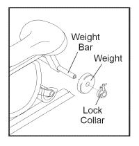
on each side of the weight bar. The total combined weight of the user and added weights should not exceed 300 pounds.
