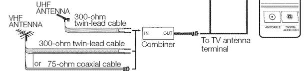
1. A 75-ohm system is generally a round cable with F-type connector that can easily be attached to a terminal without tools.
