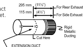
It is important to replace the ground clip after cutting the exhaust duct, (on rear exhaust model)
