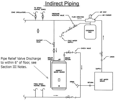
FIGURE 3 - BOILER WATER PIPING WITH ZONE CIRCULATORS
