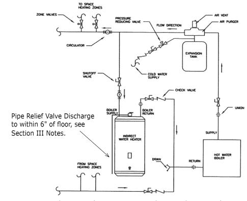
FIGURE 4 - BOILER WATER PIPING WITH ZONE VALVES
