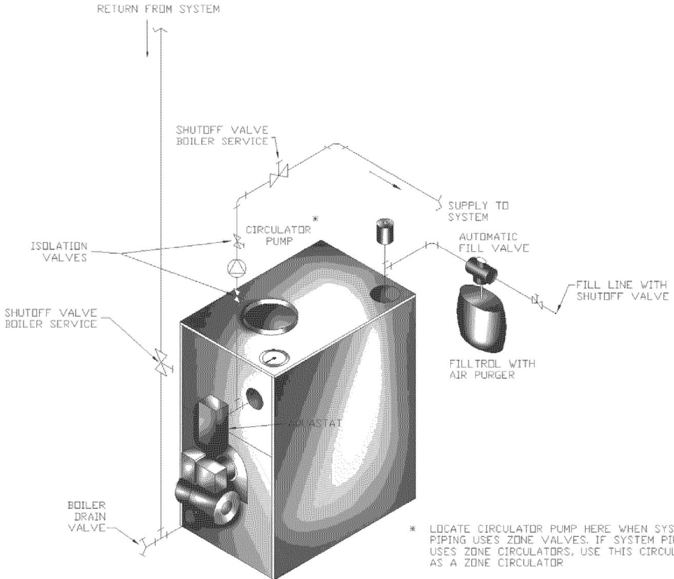
**Tankless Coil Piping Arrangement**
