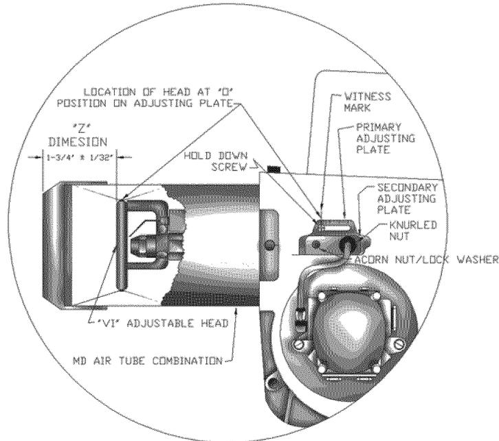
BECKETT AFG BURNER ELECTRODE ADJUSTMENTS F-HEADS
