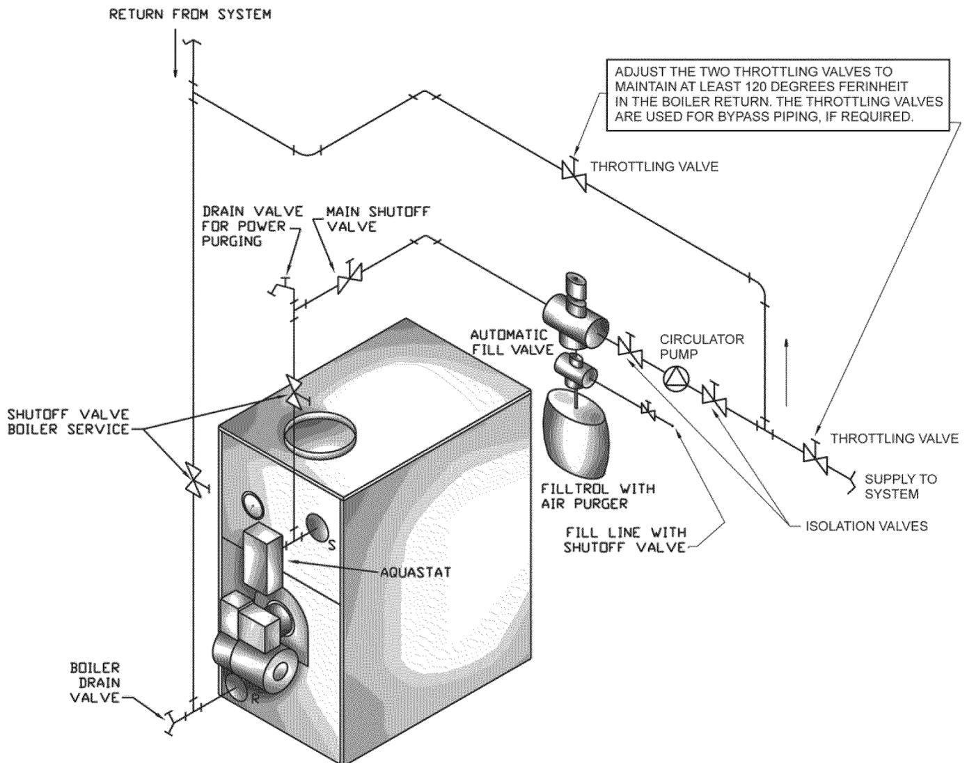
Figure 8 - System Piping Arrangement Zoning With Zone Valves
