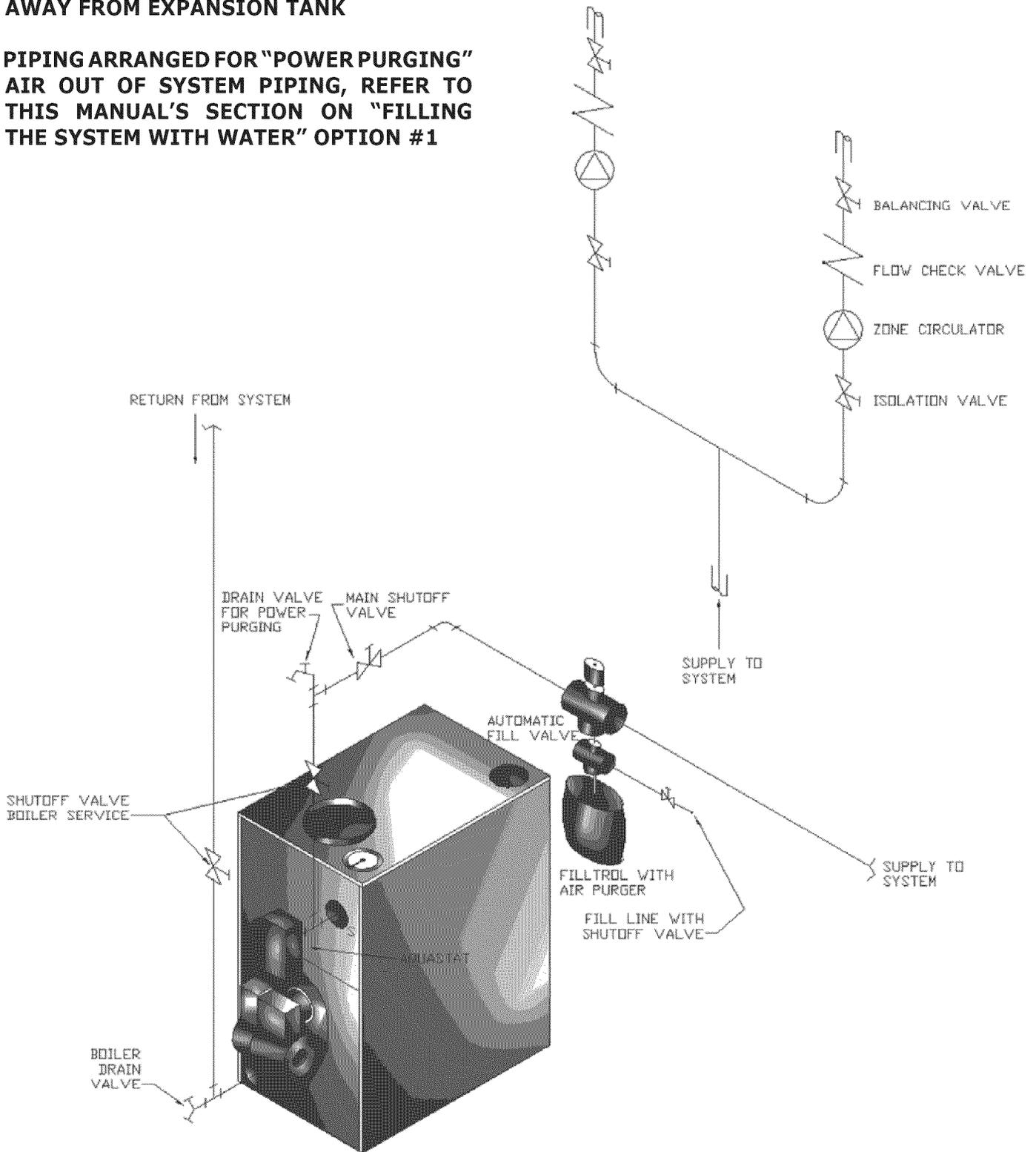
Figure 10 - System Piping Arrangement Alternate Near Boiler Piping
