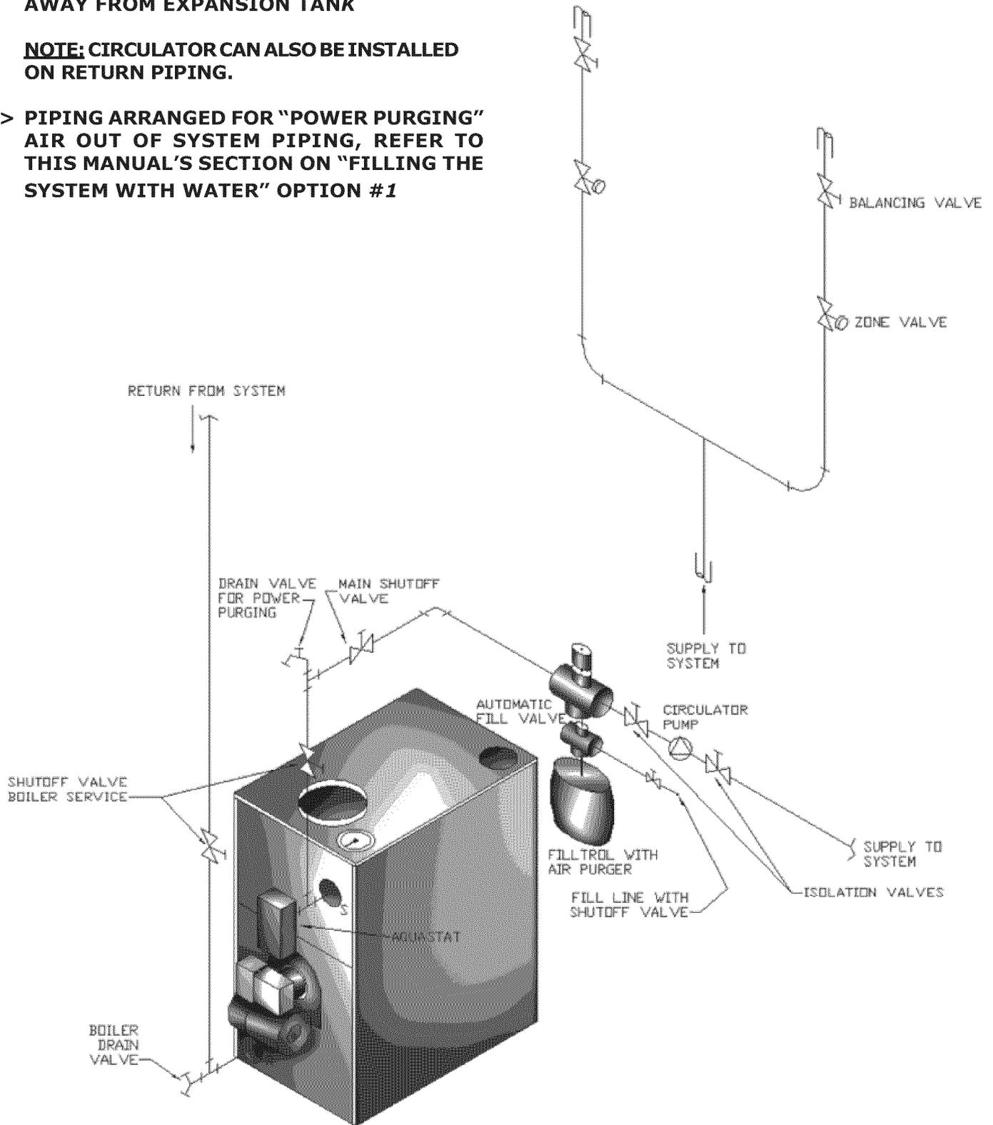
Figure 9 - System Piping Arrangement Zoning With Circulators
