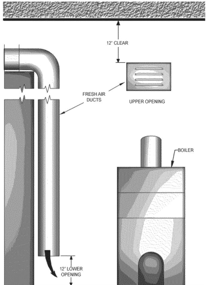
1. **Installation of boiler for new heating system,** Install all of radiation units (panels, radiators, baseboard, or tubing) and supply and return mains first. After all heating system piping and components have been installed, make final connection of system piping to boiler. It is recommended to mount circulating pump on supply side piping, such that it pumps away from expansion tank. Refer to figures on next pages.
