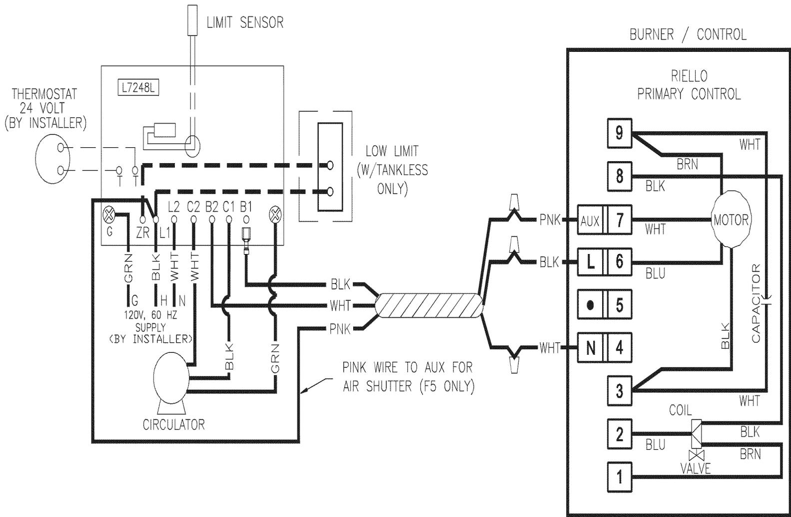
Figure 17 - Honeywell L7248L Control With Riello F5/F10 Burner
