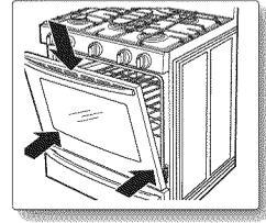
4. Completely open the oven door. If the door will not fully open, the hinge arms are not correctly inserted into the slots in the bottom of the door.
