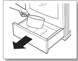
2. While supporting the drawer, pull it out until the top of the drawer sides come out of the two nylon drawer guides. Then, lift to remove the drawer.
