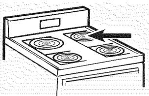
The oven is vented through an opening under the right rear surface unit.
