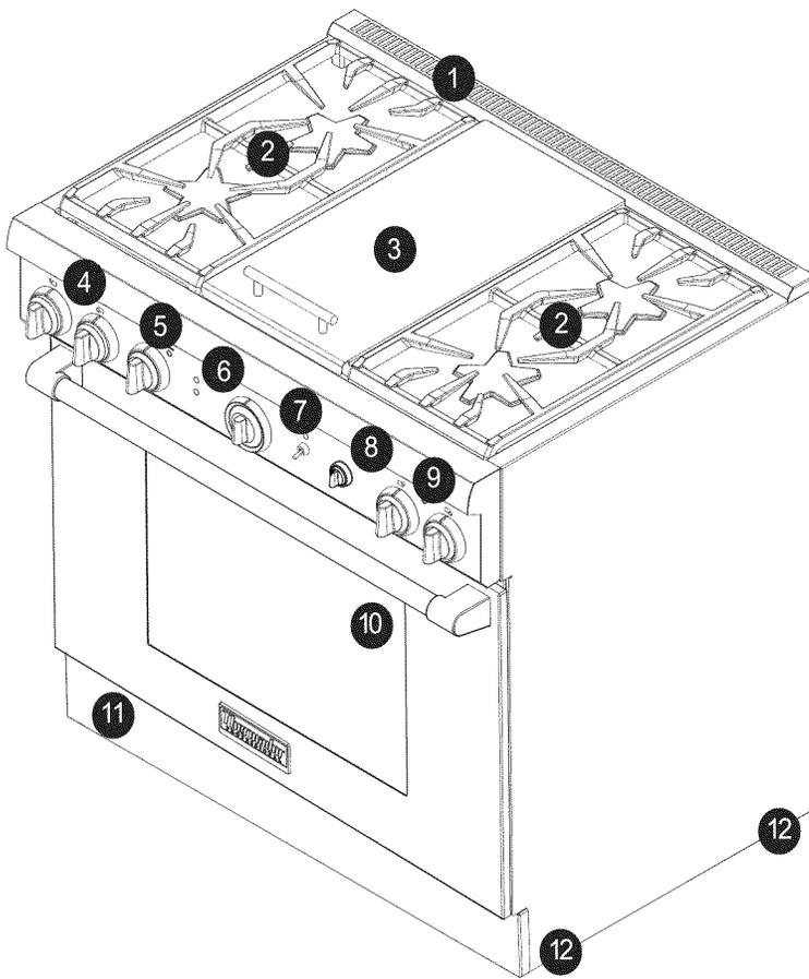
Figure 8: 36" Dual Fuel Range Identification
