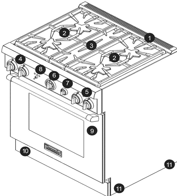
Figure 9: 30" Dual Fuel Range Identification
