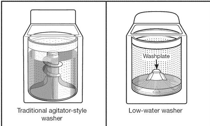
The most striking difference in your new washer is the low-water washplate wash system. The washer automatically adjusts the water level to the load size—no water level selector is needed.
