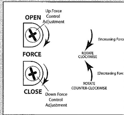
FIG. 6-5 Force Control Adjustment.
