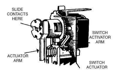
As the slide continues to be pushed inward it will contact the index wheel driver releasing the index wheel. The index wheel return spring will rotate the index wheel in a counterclockwise direction. It will continue rotating until the switch actuator arm catches a movable return stop. This stops the rotation of the index wheel for the first slide actuation.
