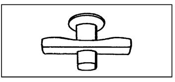
2. Remove the time adjustment peg from position "C" (as set in manufacturing) and install in position "B". See charts for additional information.
