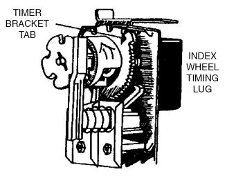
When a second movable stop is used, a third actuation of the side is possible. The third actuation will allow rotation of the index wheel counterclockwise until the index wheel timing lug contacts the timer bracket tab. Once the timing lug contacts the bracket tab, no additional drying time can be obtained.
