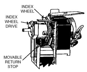
During the second coin slide actuation, the switch actuator will move into position and the index wheel will continue rotating as described in the previous actuation. It will continue rotating until either the switch actuator arm catches a second movable stop or the index wheel timing lug contacts the timer bracket tab.
