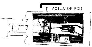
SWITCH BRACKET IS ADJUSTABLE TO ACCOMMODATE ANY COIN SLIDE.
