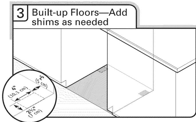
Built-up floors: If the kitchen floor is higher than the cabinet opening's floor - for example, the kitchen floor tile does not extend into the cabinet opening - add shims as needed in the area shown to bring the dishwasher up to 34" (86.4 cm) below the countertop.
