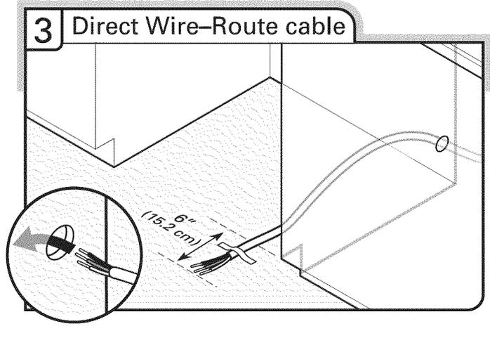
Route cable from power supply through cabinet hole (cable must extend to the right front side of cabinet opening). Tape cable to the floor in area shown. This will prohibit cable from moving when dishwasher is moved into cabinet opening.
