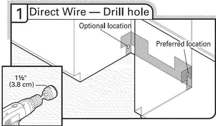
Drill a 1 1/2" (3.8 cm) hole in right-hand cabinet side or rear. See "Product and Cabinet Opening Dimensions" section.
