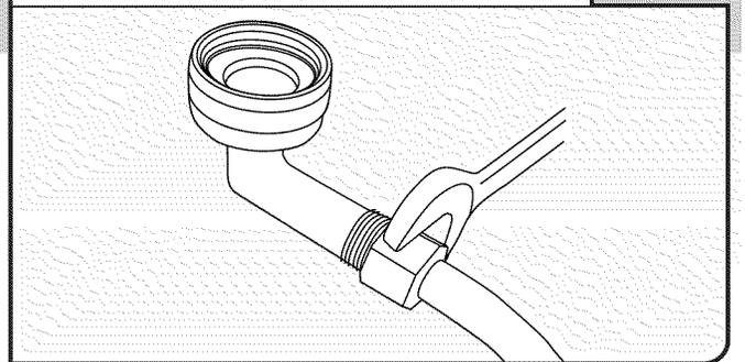
Connect the  $\frac{3}{8}$ " compression fitting to the water supply line prior to installing the unit into the cabinet opening. Attach so that the  $\frac{3}{4}$ " connection is facing upward as shown above.
