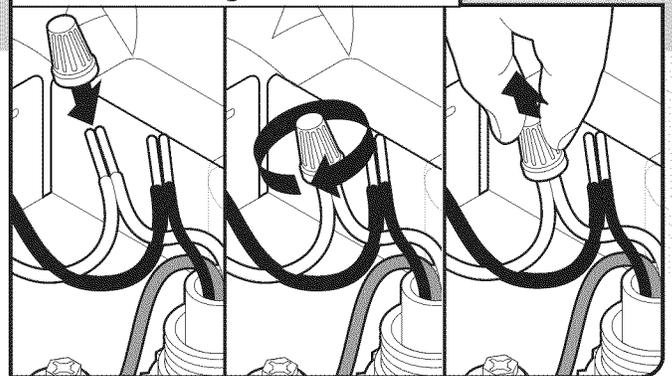
**NOTE:** Do not pre-twist stranded wire. Twist on wire connector. Gently tug on wires to be sure both are secured.
