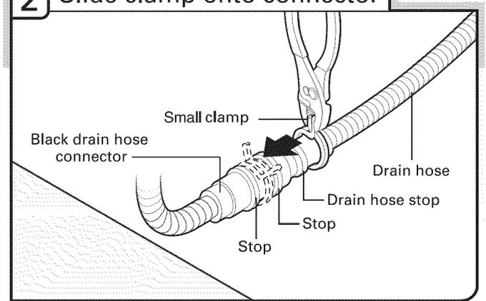
Using pliers, squeeze open the small drain hose clamp and slide onto connector between stops.
