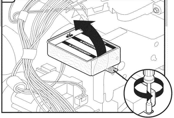
Using a  $\frac{1}{4}$ " hex head socket, nut driver or Torx® T20® screwdriver, remove terminal box cover. Retain for later use.
