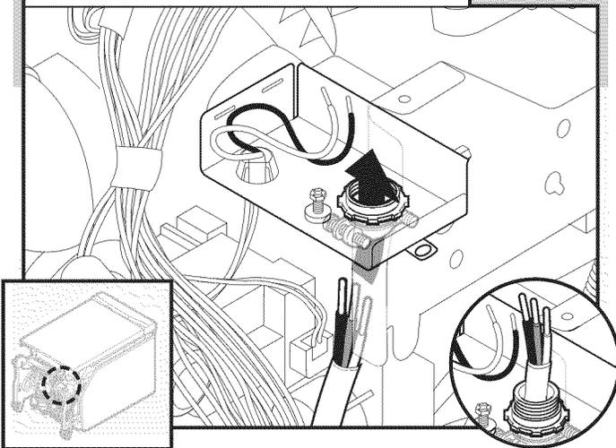
Route cord so that it does not touch dishwasher motor to lower part of dishwasher tub. Pull cord through strain relief in terminal box.
