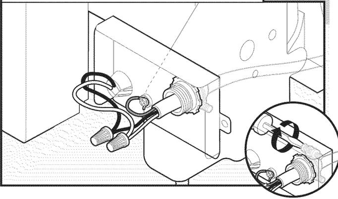
Tighten strain relief screws to secure cable.
