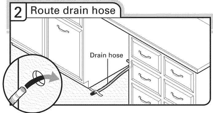
Route drain hose as shown through hole in cabinet to the front center of opening where drain connection will be made. Tape drain hose to the floor in area shown. This will prohibit it from moving when dishwasher is moved into cabinet opening.
