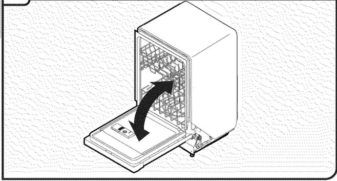
With another person holding the dishwasher to keep it from tipping, open and close the door a few times. If the door closes or falls open under its own weight, the door tension will need to be adjusted.
