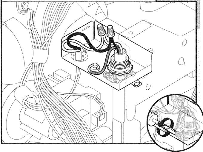
Tighten strain relief screws to secure cord.
