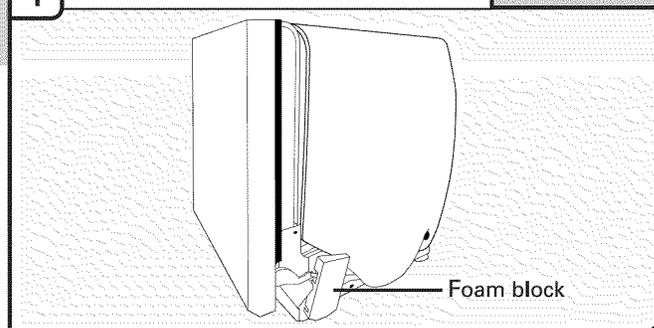
Remove and discard the foam blocks located above the front legs on each side of the dishwasher. The blocks cover the rope/link pulleys on the dishwasher.
