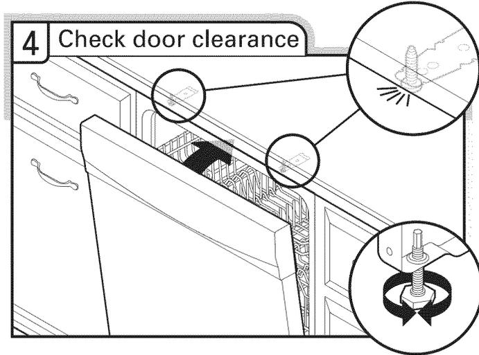
Check that top of door does not contact screws, brackets or countertop. If it does, adjust leveling legs.
