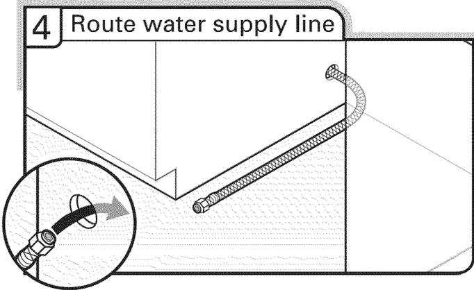
Slowly route water supply line through hole in cabinet. (If you are using copper tubing, it will bend and kink easily, so be gentle.) It should be far enough into the cabinet opening to connect it to the dishwasher inlet on the front left side of the dishwasher.
