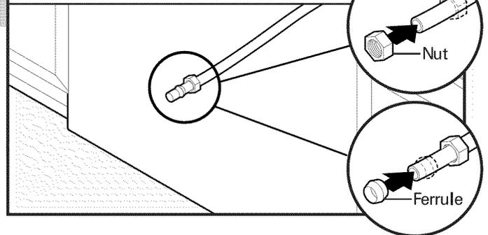
Copper tubing only: Slide nut, then ferrule, about 1" (2.5 cm) onto copper tubing.
