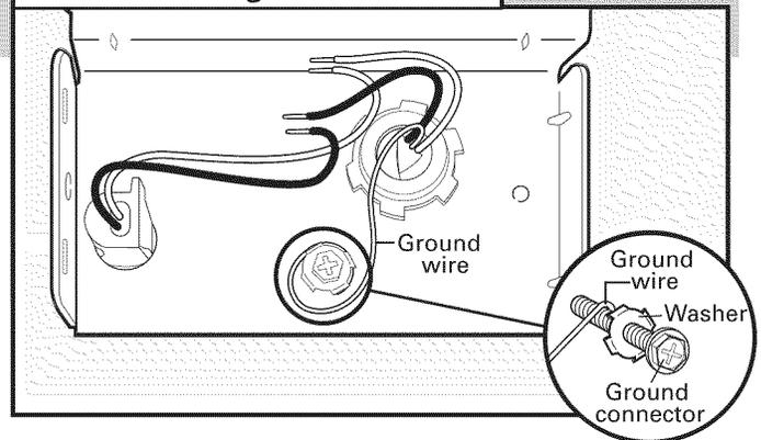
Remove the ground connector screw and place through the ring terminal of the green ground wire. Reattach and tighten the ground connector screw.
