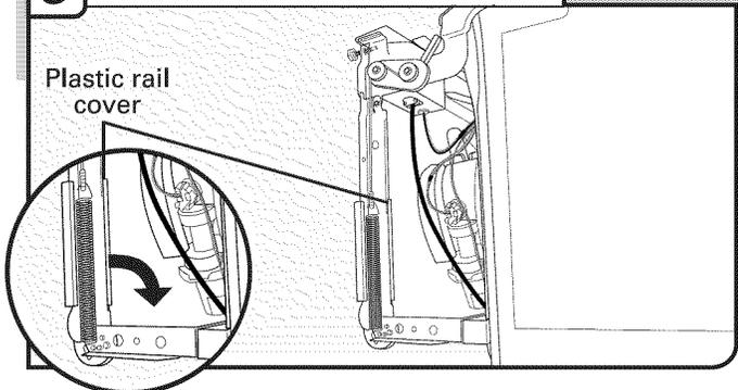
Remove and discard the plastic rail cover on each side of the dishwasher frame. To remove the plastic rail cover, push upward and back to unsnap it from the dishwasher frame.
