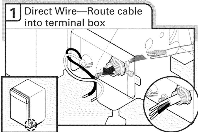
Route cable so that it does not touch dishwasher motor or lower part of dishwasher tub. Pull cable through UL Listed/CSA Approved strain relief in terminal box. Strain relief is not supplied with the dishwasher. Owner must purchase a  $\frac{7}{8}$ " screw-in type strain relief.
