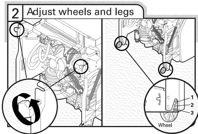
Turn both leveler legs to the same height. Put wheels in the required position determined from "Dishwasher Height Adjustment Chart."
