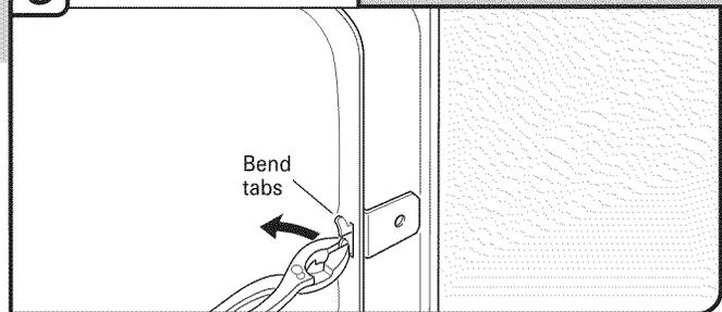
Push bracket into slot on the side of dishwasher, and bend tab in toward the side of the dishwasher so that it keeps the bracket in place. Repeat this step for the other side of the dishwasher.
