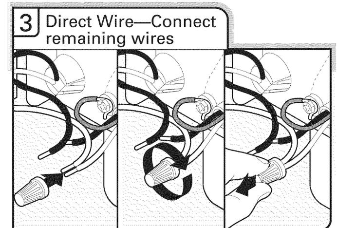
**NOTE:** Do not pre-twist stranded wire. Twist on UL listed/CSA approved wire connector. Gently tug on wires to be sure both are secured.
