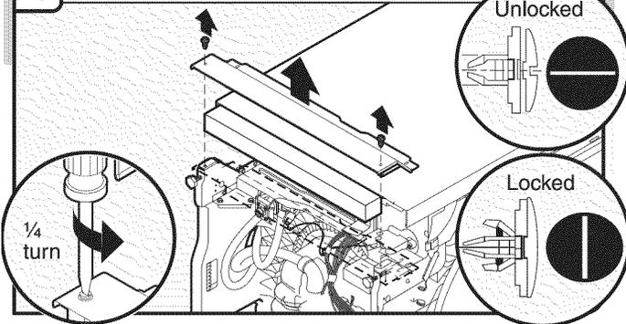
Using a flat-blade screwdriver, turn the plastic fasteners  $\frac{1}{4}$  turn counterclockwise to unlock them. Remove panel. Do not remove tech sheet from access panel.
