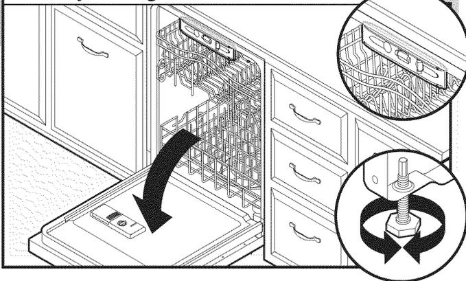
Place level against top front opening of tub. Check that dishwasher is level from side-to-side. If dishwasher is not level, adjust front legs up or down until dishwasher is level. Close the dishwasher door.
