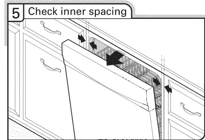
Open door and check that space between dishwasher cabinet opening and tub is equal on both sides. If spacing is not equal, loosen bracket screws secured and shift tub. Tighten bracket screws.
