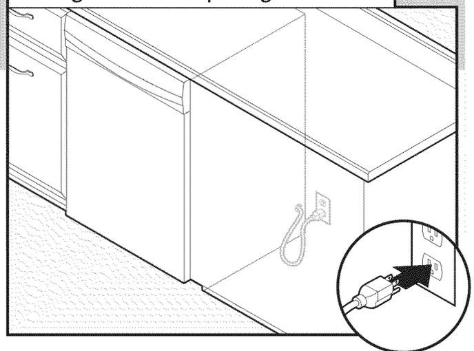
Plug into a grounded 3 prong outlet. Check that power supply cord does not touch dishwasher motor or lower part of dishwasher tub.
