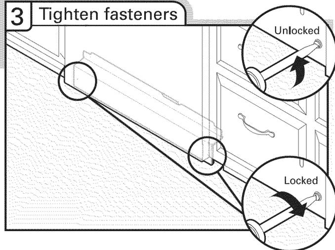
Using a flat-blade screwdriver, turn the fasteners  $\frac{1}{4}$  turn clockwise to lock into place. The fasteners slot will be straight up and down when properly locked.
