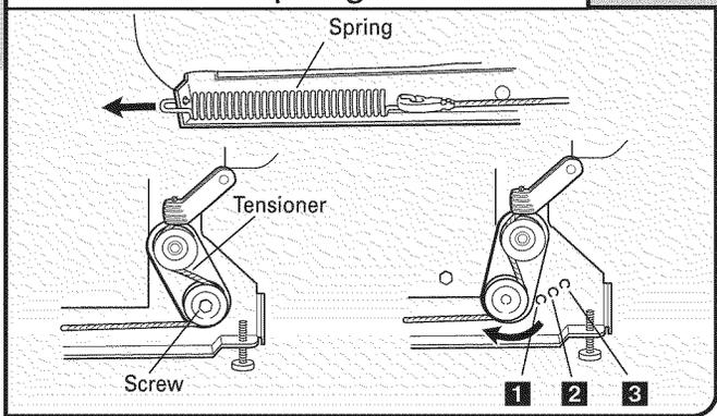
To adjust the door spring tension, unhook the spring from the rear leg of dishwasher.
