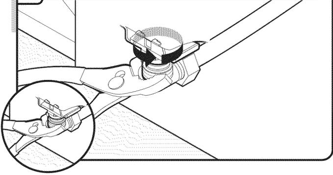
Be sure rubber washer is properly seated in fitting. Slide the 3/4" fitting up to the valve and hand tighten to avoid cross-threading. Hand tighten until the coupling is tight.
