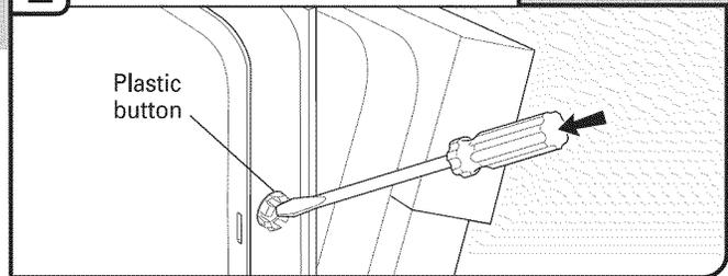
Push the plastic buttons out of the side of the tub.
