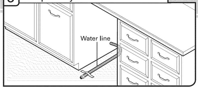
Route water line and tape it to the floor in area shown. This will keep it from moving when dishwasher is moved into cabinet opening.
