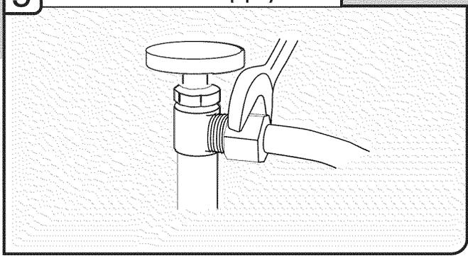
Attach the water supply line (copper tubing or flexible braided line) to the hot water line using a connection configuration that is in compliance with local codes and ordinances. The water supply to the dishwasher should have a manual shutoff valve located under the sink.
