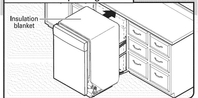
**IMPORTANT:** If wheels were removed, cover the floor when moving the dishwasher to avoid damage to the floor. Slowly move dishwasher completely into cabinet opening. Do not kink or pinch water line, drain hose, power supply cord or direct wire between dishwasher and cabinet. Remove cardboard from under dishwasher.
