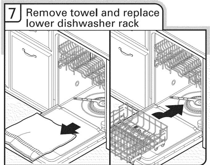
Remove towel from dishwasher. Reinstall the lower dish rack. If needed, see website for animated representation of this step. Visit [www.maytag.com/anchoring](http://www.maytag.com/anchoring) under FAQ tab.
