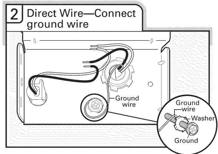
Form bare ground wire into a U-shaped hook. Wrap ground wire hook clockwise around ground connector screw and under the washer. Securely tighten ground connector screw.
