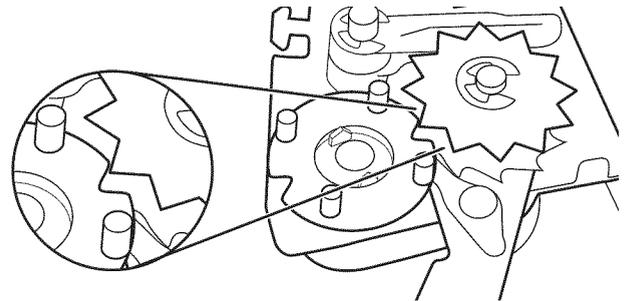
7. Press cam down in place on clock shaft. Make sure that V-shaped notch clears the ratchet tooth.
