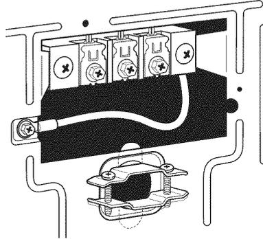
2. Insert power cord into strain relief.
