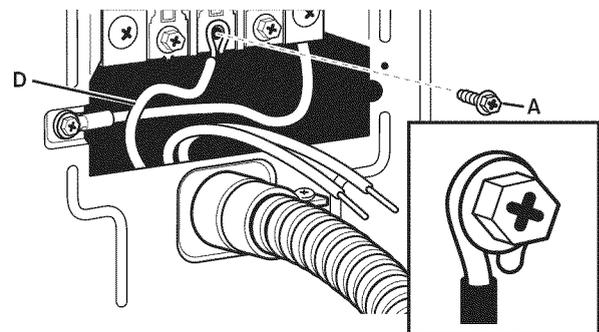
3. Connect remaining wires under outer terminal block screws (F). Squeeze hooked ends together and tighten screws. Finally, reinstall terminal block to dryer rear panel. Secure cover with hold-down screw.
