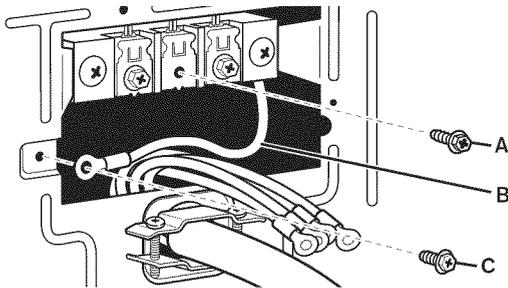
2. Connect neutral ground wire (B) and neutral wire (white or center wire) (D) of power supply cord/cable under center terminal block screw (A). Tighten screw.
