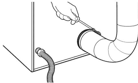
4. Make sure the vent is secured to exhaust hood with a 4" (102 mm) clamp.
