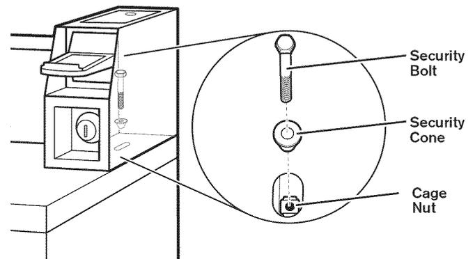
**NOTE:** Installing the security bolt provides added security, but will add to the service time when the top needs to be removed for servicing the dryer.
