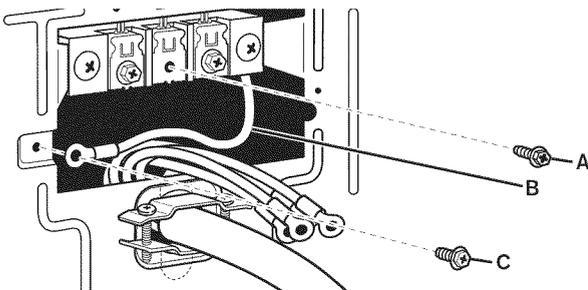
2. Connect neutral ground wire (B) and neutral wire (white or center wire) (D) of power supply cord under center terminal block screw (A). Tighten screw.
