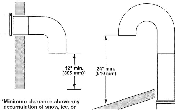
If main vent travels vertically through the roof, rather than through wall, install a 180° sweep elbow on end of vent at least 2 ft. (610 mm) above surface of roof.
