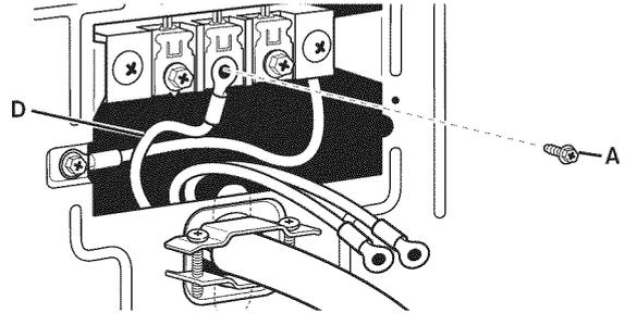
3. Connect remaining wires under outer terminal block screws (F). Tighten screws. Finally, reinstall terminal block to dryer rear panel. Secure cover with hold-down screw.
