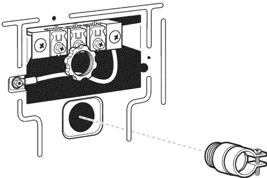
2. Insert conduit into strain relief and tighten clamp.
