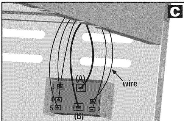
**NOTE:** Switch terminals are larger than electrode terminals and should only be installed in location shown as (A), (B).
