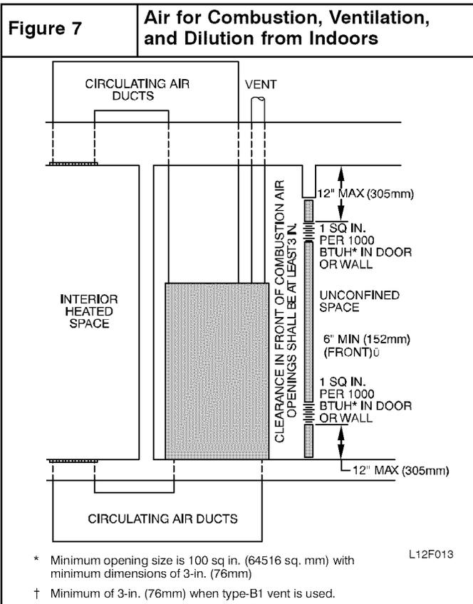
3. In spaces that use the **Indoor Combustion Air Method**, infiltration should be adequate to provide air for combustion, permanent ventilation and dilution of flue gases. However, in buildings with unusually tight construction, additional air **MUST** be provided using the methods described in the **Outdoor Combustion Air Method** section.
