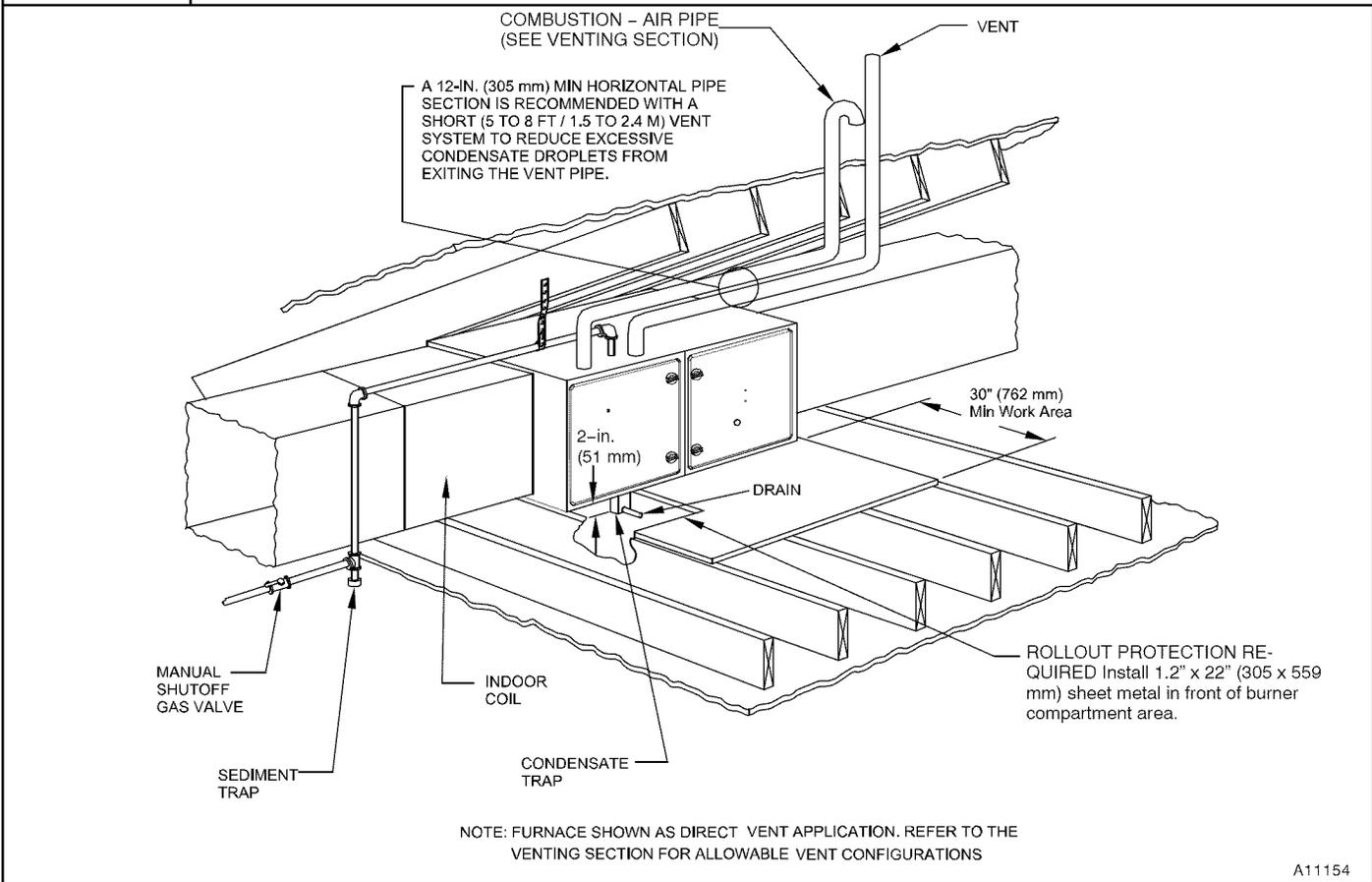
NOTE: FURNACE SHOWN AS DIRECT VENT APPLICATION. REFER TO THE VENTING SECTION FOR ALLOWABLE VENT CONFIGURATIONS
