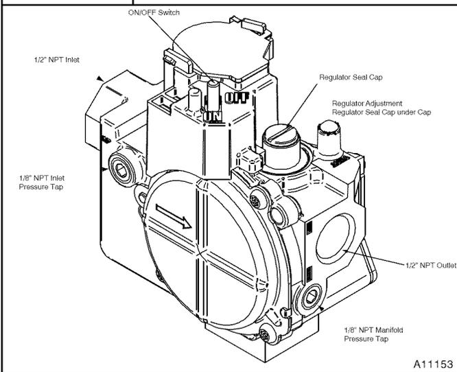
If pressure exceeds 0.5 psig (14-in. w.c.), gas supply pipe must be disconnected from furnace and capped before and during supply pipe pressure test. If test pressure is equal to or less than 0.5 psig (14-in. w.c.), turn off electric shutoff switch located on furnace gas control valve and accessible manual equipment shutoff valve before and during supply pipe pressure test. After all connections have been made, purge lines and check for leakage at furnace prior to operating furnace.
