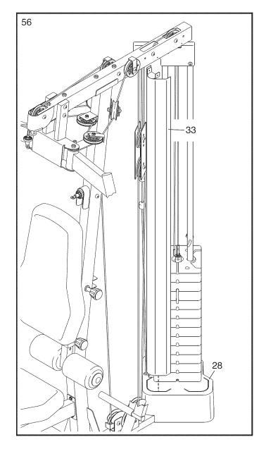
57. Attach the top of the Center Shroud (33) to the Top Frame (6) with two ST4.2 x 19mm Screws (90).
