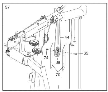
38. Route the Low Cable (43) under a Pulley (69).
