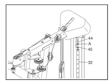
Do not overtighten the cables. If the cables are overtightened, the top weight will be lifted off the weight stack. If a cable tends to slip off the pulleys often, it may have become twisted. Remove the cable and reinstall it. If the cables need to be replaced, see the back cover of this manual.
