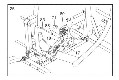
26. Route the Low Cable (43) around a Pulley (69) and then route it through the bracket in the Base (1) as shown.
