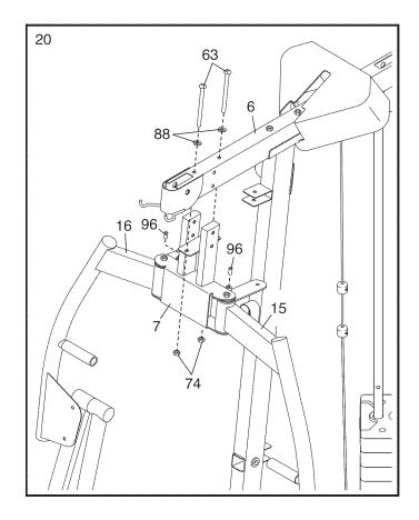
21. Finish attaching the Butterfly Frame (7) to the Top Frame (6) with two M10 x 117mm Bolts (64), four M10 Washers (88), and two M10 Locknuts (74).
