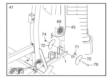
42. Route the Low Cable (43) under a Pulley (69).
