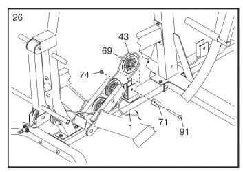
27. Route the Low Cable (43) over a Pulley (69).
