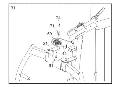
32. Route the High Cable (44) around a Pulley (69).
