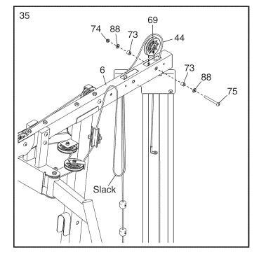
36. Insert a Pulley (69) under the High Cable (44) in the location shown.
