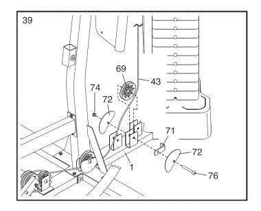
40. Route the Low Cable (43) over a Pulley (69).
