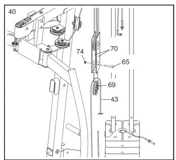
41. Route the Low Cable (43) under a Pulley (69).
