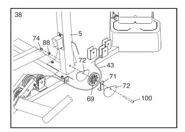
39. Route the Low Cable (43) under a Pulley (69).
