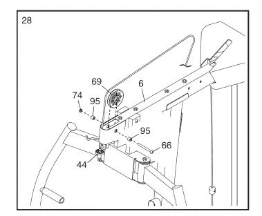
29. Route the High Cable (44) over a Pulley (69).
