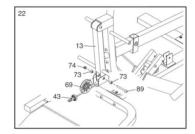
23. Route the Low Cable (43) over a Pulley (69) and through the Leg (10).
