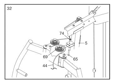
33. Route the High Cable (44) around a Pulley (69).
