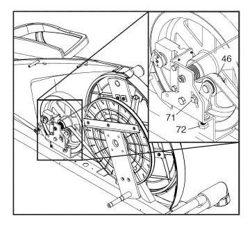
When the Drive Belt (46) is tight, tighten the Pivot Screw (71).
