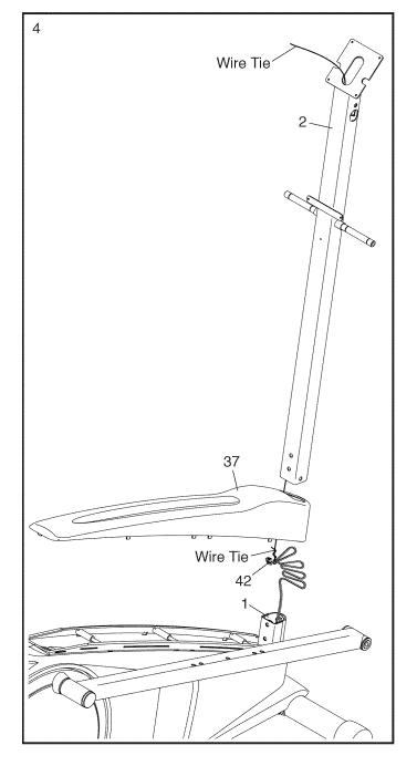
5. **Tip: Avoid pinching the Main Wire (42).** Slide the Upright (2) onto the Frame (1).
