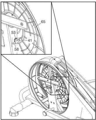
Next, rotate the Pulley (65) until a Magnet (41) is aligned with the Reed Switch (58). Slide the Reed Switch slightly toward or away from the Magnet. Then, retighten the M4 x 16mm Screw (53).
