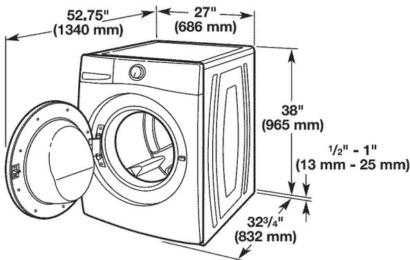
All dimensions show recommended spacing allowed, except for closet door ventilation openings which are the minimum required.
