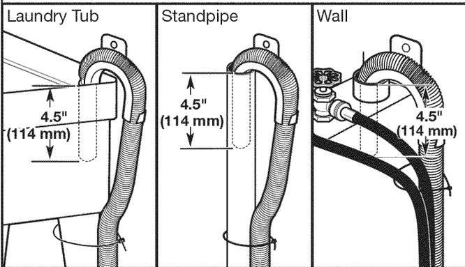
Secure drain hose to laundry tub leg, drain standpipe, or inlet hoses for wall standpipe with cable tie.
