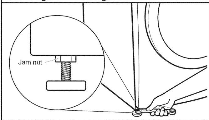
When washer is level and all four feet are firmly in contact with the floor, use a 9/16" or 14 mm open-end or adjustable wrench to turn jam nuts counterclockwise on leveling feet tightly against washer cabinet.
