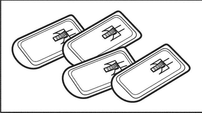
Close bolt holes on cabinet back with four transport bolt hole plugs included with washer parts.
