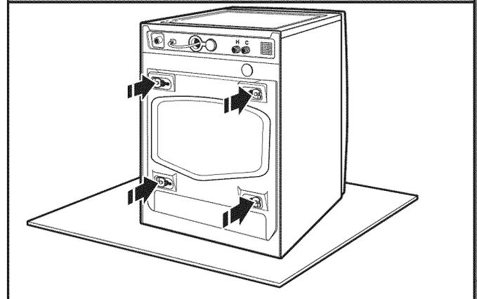
Locate four transport bolts on rear of washer.
