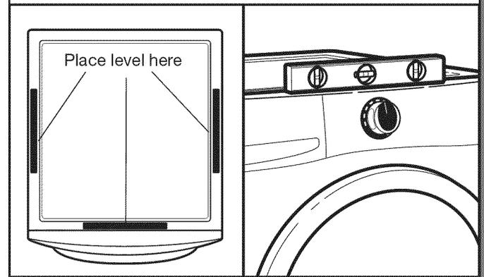
Remove cardboard from beneath washer. Place a level on top edges of washer, checking each side and front. If not level, tip washer and adjust feet up or down as shown in steps 18 and 19, repeating as necessary.
