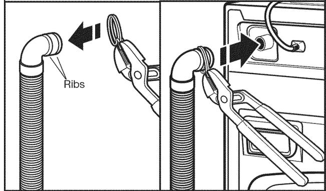
If clamp is not already in place on elbow end of drain hose, squeeze clamp with pliers and slide it over end of hose, centering it between the ribs, as shown. Squeeze clamp with pliers and slide elbow end of drain hose onto drain port and secure with clamp.
