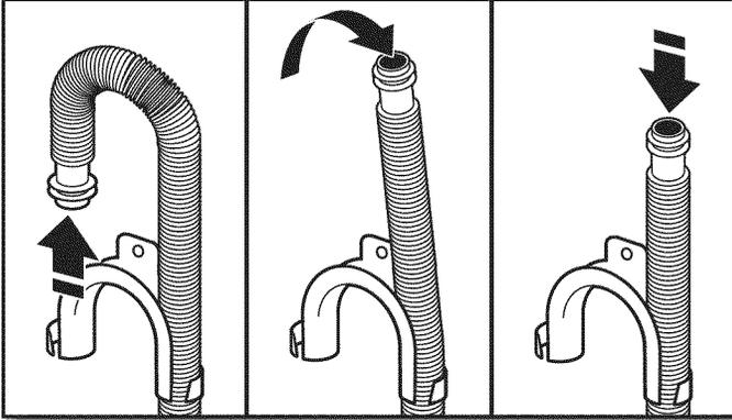
For floor drain installations, you will need to remove the drain hose form from the end of the drain hose. You may need additional parts with separate directions. See "Alternate Parts".
