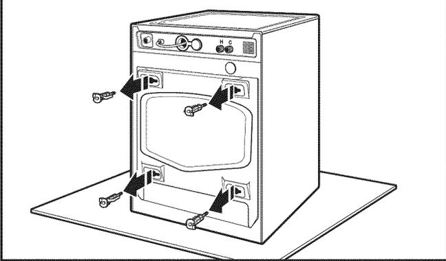
Loosen bolts with a 1/2" (13 mm) wrench. Slide each bolt and spacer to center of hole. Pull bolts and plastic spacers from back of washer. Discard bolts and spacers.
