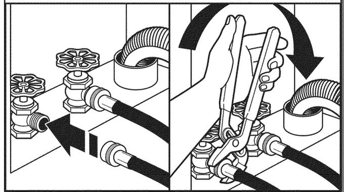
Attach the hose labeled hot to hot water faucet. Screw on coupling by hand until it is seated on washer. Use pliers to tighten couplings an additional two-thirds turn. Repeat this step with the hose labeled cold for the cold water faucet. Both hoses must be connected for washer to work properly.
