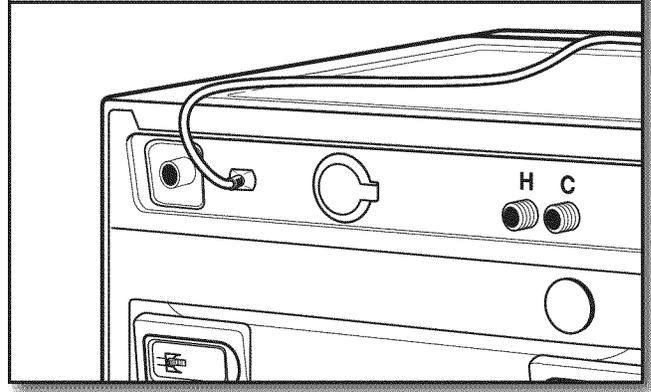
Remove the yellow shipping strap from the cord. Gently place power cord over top of washer to allow free access to back of washer.
