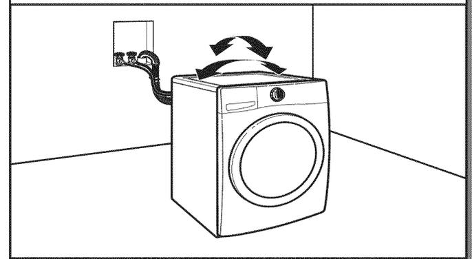
Grip washer from top and rock back and forth, making sure all four feet are firmly on floor. Repeat, rocking washer from side to side. If washer rocks, go to step 18 and adjust leveling feet. If all four feet are in firm contact with floor, go to Step 19.
