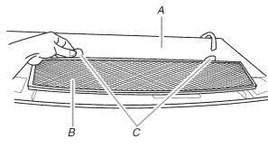
A. Top of microwave oven B. Vent screen C. Rings
