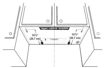
**5.** Cut the  $1\frac{1}{2}$ " (3.8 cm) diameter hole at the circular shaded area "G" on the template. This hole is for the power supply cord.
