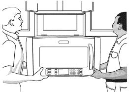
**3.** Using 2 or more people, lift microwave oven and hang it on support tabs at the bottom of mounting plate.
