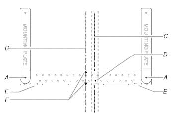
NOTE: If wall stud is within 6" (15.2 cm) of the vertical centerline (see "Mark Rear Wall" section), only recirculation or roof venting installation can be done.
