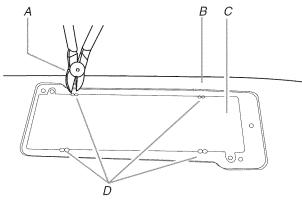
A. Diagonal wire cutting pliers B. Top of microwave oven C. Roof damper vent cover D. Perforations
