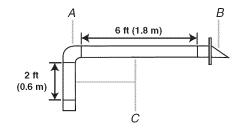
A. One 3 ¼" x 10" (8.3 x 25.4 cm) 90° elbow = 25 ft (7.6 m) B. 1 wall cap = 40 ft (12.2 m) C. 2 ft (0.6 m) + 6 ft (1.8 m) straight = 8 ft (2.4 m)
