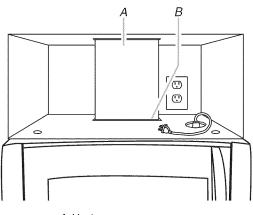
A. Vent B. Damper assembly (under vent)
