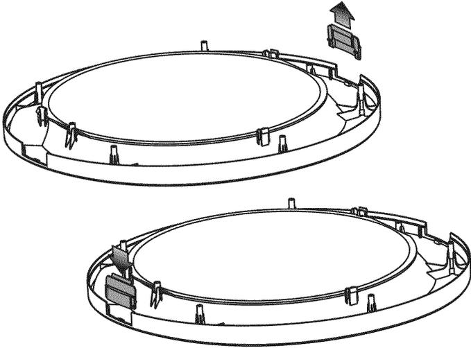
2. Rest the opening of the inner door at a 90 degree angle on the "shoulders" of the hinge cutout gate. Pivot the inner door down onto the outer door.
