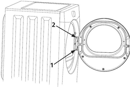
3. Supporting door with both hands, squarely lift door and hinge upward approximately 3/8" (10 mm) so "T" post on back of hinge can slide out through "T" slot on front panel.
