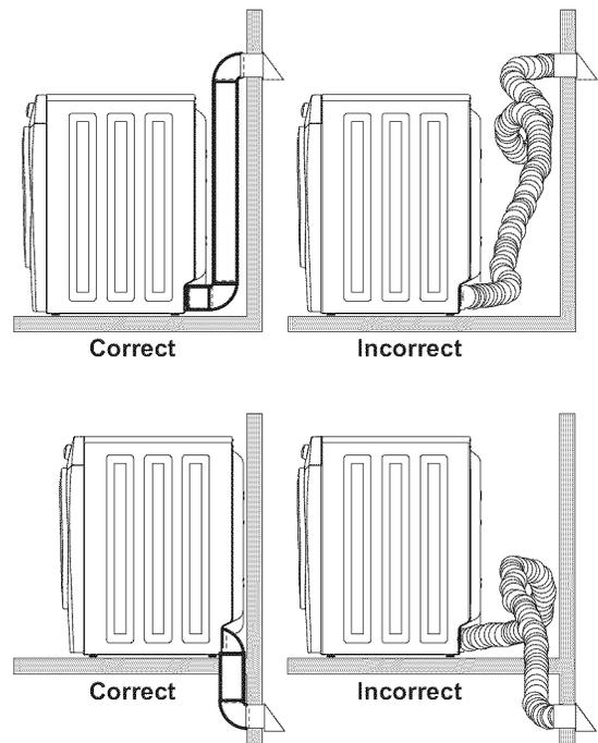
If your present system is made up of plastic duct or metal foil duct, replace it with a rigid or semi-rigid metal duct. Also, ensure the present duct is free of any lint prior to installing dryer duct.
