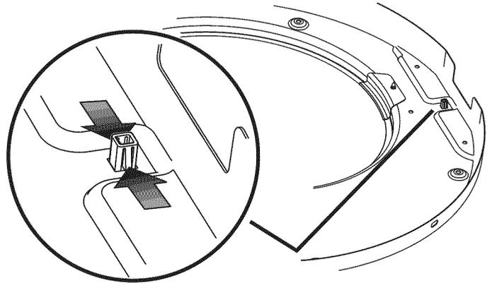
5. Carefully remove the 2 round plugs from the inner door and move them to the opposite holes and reinstall.
