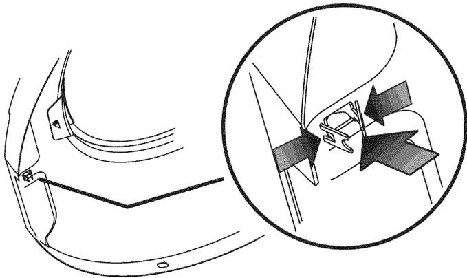
3. Turn the inner door assembly back over and locate the 2 pan head hinge screws. Remove and save the 2 screws and separate the hinge from inner door assembly.
