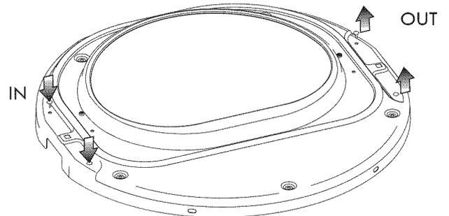
6. Rotate the hinge and move it to the opposite side of the inner door. Attach it with the 2 pan head screws removed previously. Reinstall plastic plug in the square hole next to the hinge.
