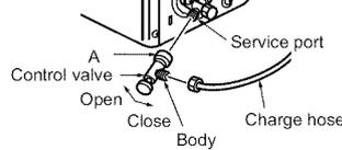
When attaching the control valve to the service port, make sure that the valve core is in closed position, and then tighten part A. Do not tighten part A or turn the body when valve core is in open position.
