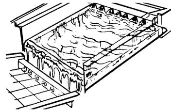
2. When the desired thickness is reached, the ice sheet is released and slides onto a cutter grid. The grid divides the sheet into individual cubes.
