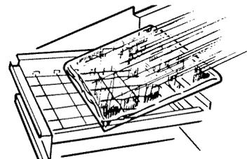
3. The water containing the rejected minerals is drained after each freezing cycle.
