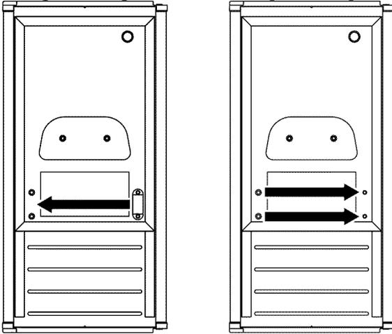
3. Push the hole plugs into place on the opposite side of the door.
