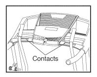
To measure your heart rate, stand on the foot rails and hold the metal contacts on the console. Avoid moving your hands. When your pulse is detected, a heart symbol in the lower right display will flash each time your heart beats, one or two dashes will appear, and then your heart rate will be shown. For the most accurate heart rate reading, continue to hold the contacts for about 15 seconds.
