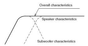
When the subwoofer's output level is incorrect
