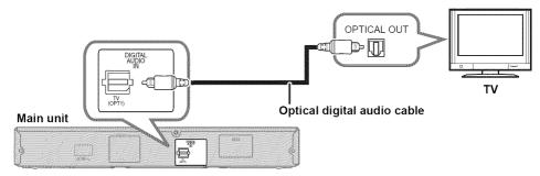
• When you use the optical digital audio cable, insert the tip correctly into the terminal.
