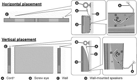
\* If the cord cannot be threaded through the holes, try bending the cord in 2 locations, about 10 mm (13/32") apart from the tip, at an angle of 45° (as illustrated above).
