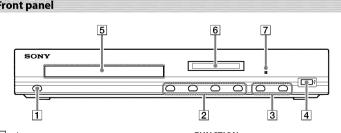
1 I/U (on/standby) Turns on the unit, or sets it to standby
