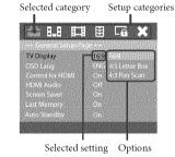
[4:3 Pan Scan]: Displays a full-height picture on the entire screen, with trimmed sides.
