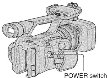
**1** While pressing the green button, slide the POWER switch.
