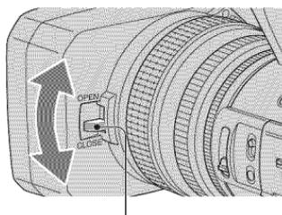
Move the lens cover lever to OPEN to open the lens cover, and move the lever to CLOSE to close the lens cover.
