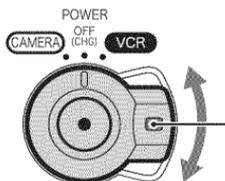
Press and hold the green button when you slide the POWER switch from OFF (CHG).
