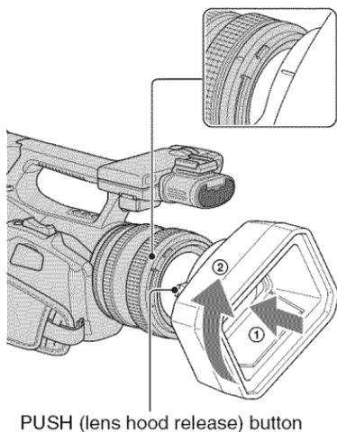
Align the marks on the lens hood to those on the camcorder, and turn the lens hood in the direction of the arrow ②.
