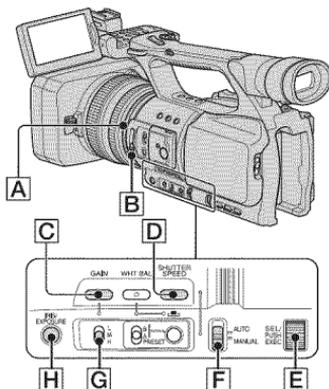
You can adjust the image brightness by adjusting the iris, the gain or the shutter speed or by reducing the light volume with the ND filter **B**. Also, when [EXPOSURE] is assigned to the iris ring, you can adjust the iris, gain and shutter speed with the iris ring **A**. You can assign [IRIS] or [EXPOSURE] to the iris ring **A** from [IRIS/EXPOSURE] of the (CAMERA SET) menu (p. 66). The default setting is [IRIS].
