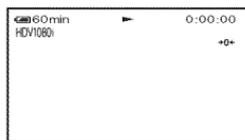
If the tape counter is not displayed, press the DISPLAY button **G**.
