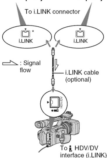
\* An i.LINK jack which is compatible with HDV1080i specification is required.
