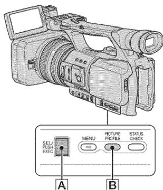
You can customize the picture quality by adjusting picture profile items such as [COLOR LEVEL] and [SHARPNESS]. Connect your camcorder to a TV or monitor, and adjust the picture quality while observing the picture on the TV or monitor screen.
