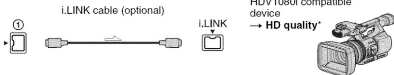
• i.LINK jack which is compatible with HDV1080i specification is required on the external device.
