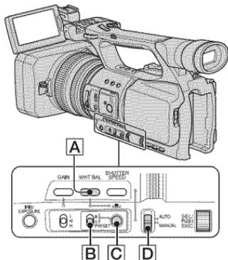
You can adjust and fix the white balance according to the lighting conditions of recording environment. You can store white balance values in memory A (**A**) and memory B (**B**), respectively. Unless a white balance is readjusted, values will remain even after the power has been turned off.
