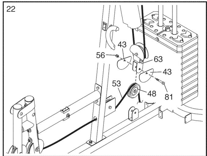
23. Route the Low Cable (53) under a Thick Pulley (48).
