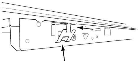
*Insert bottom of mounting clip into bottom of pocket and push top over top of pocket to snap into place.*
