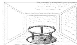
4. Place the glass tray securely in the center of the pre-assembled roller ring.
