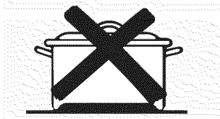
Pans with rounded, curved, ridged or warped bottoms are not recommended.
