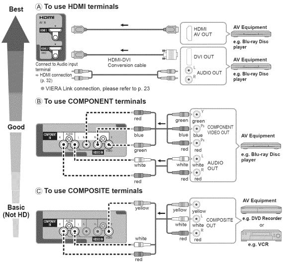
The Green terminal is shared for both the COMPONENT and COMPOSITE (VIDEO IN) connection. When using COMPOSITE (VIDEO IN) connection, the Yellow connector (Video) should be inserted into Green connection. (Watching content from external devices (p. 16))
