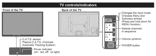
Remote control sensor within about 23 feet (7 meters) in front of the TV set · An image of the control panel is displayed on the screen while using it.
