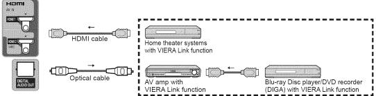
No optical cable is necessary when connecting a Home Theater supporting "HDAVI control 5" with an HDMI cable. Audio will be supported via ARC (Audio Return Channel) (p. 22)
