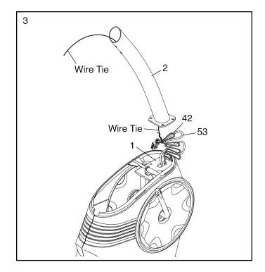
4. **Tip: Avoid pinching the wires.** Set the Upright (2) on the Frame (1).
