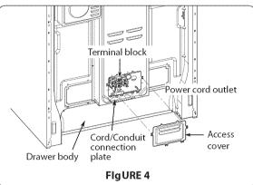
The Cord/Conduit connection plate is used for the installation of power cord or conduit. For power cord, install it with the connection plate as INSTALLED. For conduit, remove the connection plate located below the rear of the drawer body and use the conduit hole  $(1 \ 1/8'')$  instead of power cord hole  $(1 \ 3/8'')$ . (Refer to Figure 5 and 6.)
