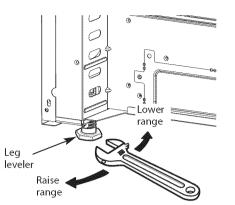
Use a level to check your adjustments. Place the level diagonally on the oven rack, and check each direction for level.
