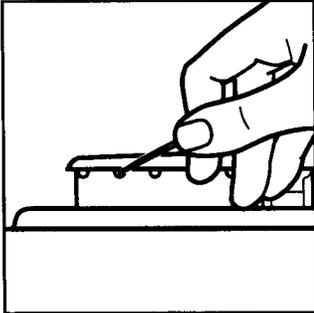
5. After cleaning the gas tube opening and ports, replace the burner caps. To replace the burner caps, make sure the alignment pins are properly aligned with the burner base.
