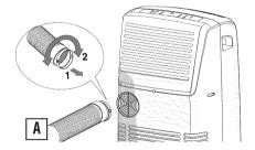
Screw the window outlet **17** to the other end of the exhaust hose. (see fig. **B**).
