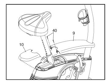
Next, locate the Reed Switch (21). Loosen, but do not remove, the M4 x 16mm Screw (40).
