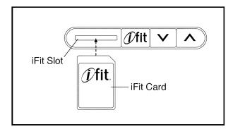
Next, select the desired workout on the iFit card by pressing the increase and decrease buttons next to the iFit slot.
