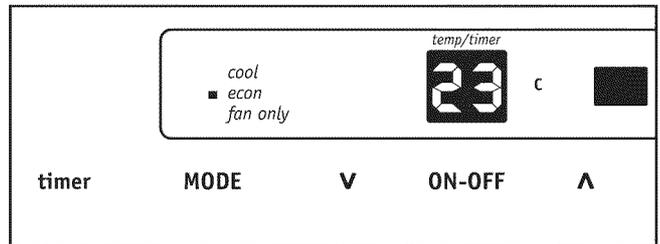
Note: In this mode, the fan will continue to run for 1 minute after the compressor shuts off. The fan then cycles on for 20 seconds at 10 minute intervals until the room temperature is above the set temperature, at which time the compressor turns back on.
