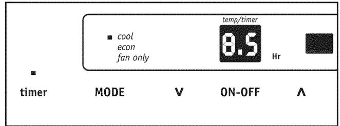
Note: For Delay Stop, the unit must be in the On position.
