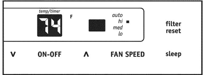
Note: The control is capable of displaying temperature in degrees Fahrenheit or degrees Celsius.
