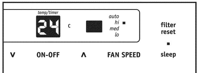
Note: In this mode the selected temperature will increase by 1 °C 30 minutes after the mode is selected. The temperature will then increase by another 1 °C after an additional 30 minutes. This new temperature will be maintained for 7 hours before it returns to the originally selected temperature. This ends the "Sleep" mode and the unit will continue to operate as originally programmed. The "Sleep" mode program can be cancelled at any time during operation by again pressing the "Sleep" button.
