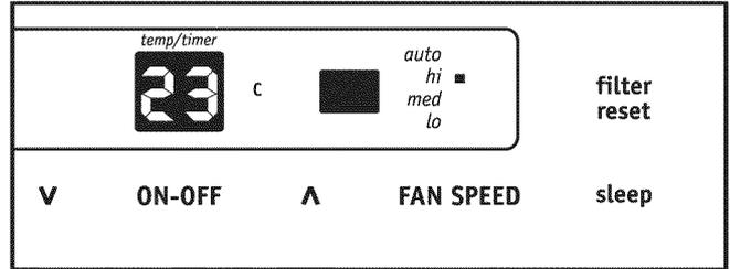
Note: Tap or hold either up ( **▲** ) or down ( **▼** ) button until the desired temperature is seen on the display. This temperature will be automatically maintained anywhere between 16 °C (60 °F) and 32 °C (90 °F) . If you want the display to read the actual room temperature. See "To Operate on Fan Only" section on Page 7.
