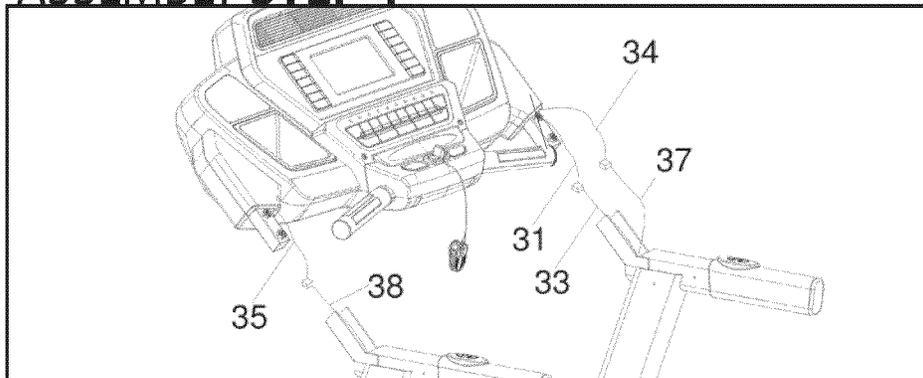
1. Connect the Speed Switch Cable (37) to the upper Speed Cable (34).
