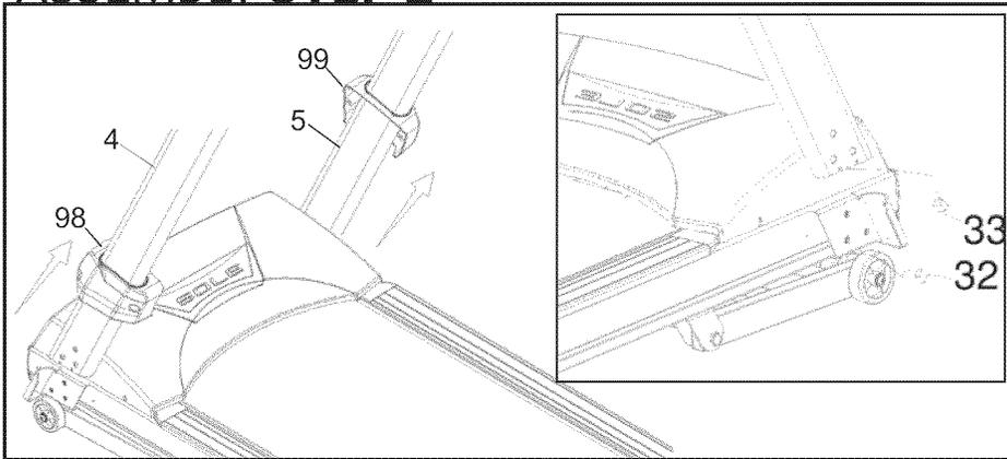
1. Slide the console mast tube covers (99 onto 5 & 98 onto 4) onto the left and right console mast tubes. Make sure the holes face the outside on each side. Connect the lower Computer Cable (32) with the middle Computer Cable (33).
