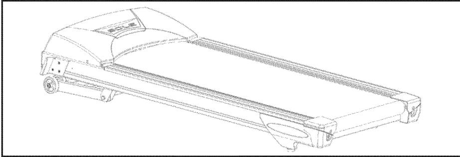
1. Remove the treadmill base frame from the carton and lay it aside on firm, level ground.
