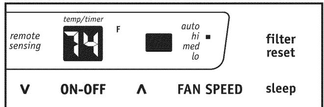
Note: The control is capable of displaying temperature in degrees Fahrenheit or degrees Celsius.
