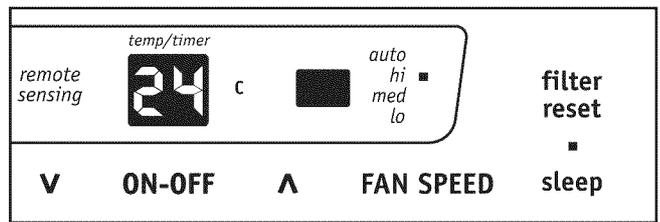
Note: In this mode the selected temperature will increase by 1 °C 30 minutes after the mode is selected. The temperature will then increase by another 1 °C after an additional 30 minutes. This new temperature will be maintained for 7 hours before it returns to the originally selected temperature. This ends the "Sleep" mode and the unit will continue to operate as originally programmed. The "Sleep" mode program can be cancelled at any time during operation by again pressing the "Sleep" button.
