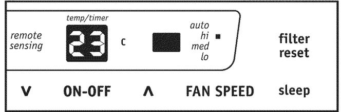
Note: Tap or hold either up ( **A** ) or down ( **V** ) button until the desired temperature is seen on the display. This temperature will be automatically maintained anywhere between 16 °C (60 °F) and 32 °C (90 °F) . If you want the display to read the actual room temperature. See "To Operate on Fan Only" section on Page 7.
