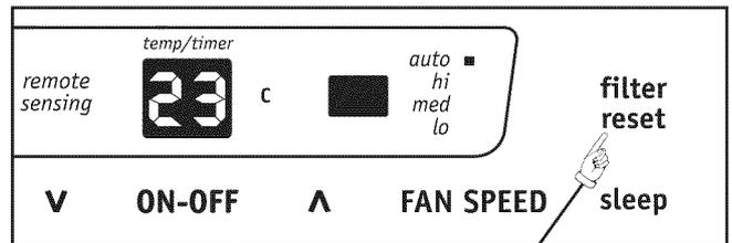
Note: This feature is a reminder to clean the Air Filter (See Care and Cleaning) for more efficient operation. The LED (light) will illuminate after 250 hours of operation. To reset after cleaning the filter, press the "Filter Reset" button and the light will go off.
