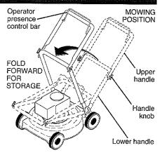
2 POSITION / "ADJUSTABLE" HANDLES When setting you handles up from the storage position, the lower handle will automatically lock into mowing position.
