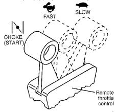
MODELS WITH FIXED SPEED ENGINES Engine speed was set at the factory for optimum performance. Engine speed is not adjustable.
