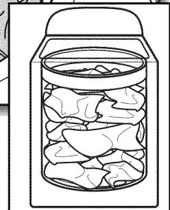
Load garments in loose heaps evenly around the washplate. Do not load garments directly over the center of the washplate; when loaded, the center of the washplate should be visible. Try mixing different sized garments to reduce tangling.
