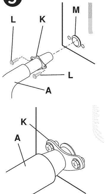
Connect drain hose **A** to drain opening on back of washer. Push hose **A** into opening using your hands until clamp **K** on drain hose is about 1/2" from washer back. Insert 2 screws **L** through holes in clamp **K** and into holes at either side of drain opening. Tighten screws with screwdriver or 1/4" nut driver. Clamp **K** will be bowed and about 1/4" from washer back after screws are tightened.
