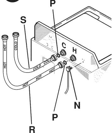
Remove electrical cord **N** from storage before installing water hoses. If not installed, install rubber washer **P** in one end of hot water hose **R**. Thread hot water hose **R** onto connection labeled **H** at top rear of washer. Hand tighten, plus an additional 1/8 turn with pliers.
