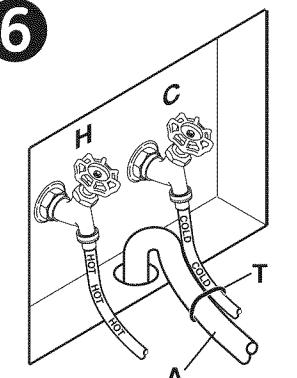
NOTE: If longer drain hose is required, order drain hose extension kit, GE part number WH49X301. Connect additional drain hose (contained in kit) to original hose with hose clamp (contained in kit).
