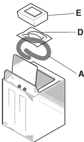
After the machine is in the home, remove outside packing material/carton from washer.
