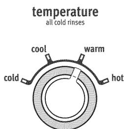
Once you select a cycle, select the desired wash temperature by turning the Temperature knob to the desired setting.
