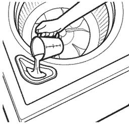
**IMPORTANT:** Do not add detergent to CLEAN WASHER cycle. Do not use more than recommended amount of bleach to avoid damaging product over time.
