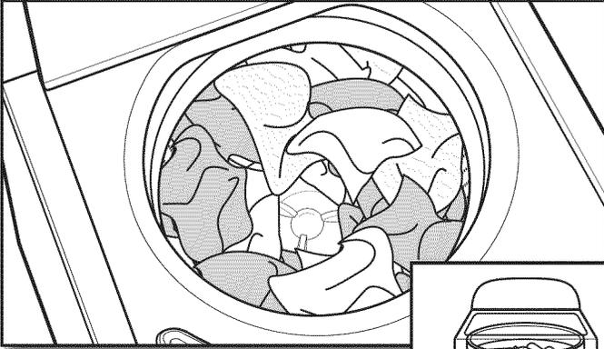
Load garments in loose heaps evenly around the washplate. Do not load garments directly over the center of the washplate; when loaded, the center of the washplate should be visible. Try mixing different sized garments to reduce tangling.
