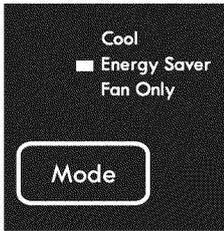
You will save energy usage in this mode. The compressor and motor will turn off once the room is at the desired temperature. The air will be sampled for 20 seconds every 10 minutes until the room is above the set temperature, at which point the compressor turns back on and the fan runs. The entire process is now repeated.
