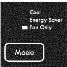
Use Fan Only function to circulate room air without air conditioner cooling. You can use any fan speed you prefer and the actual room temperature will be displayed in the DISPLAY.
