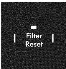
After 250 hours of operation, the Filter Reset LED will light. This is a reminder to clean the filter housed behind the front panel to keep the unit operating efficiently. Pressing the **FILTER RESET** button for 3 seconds will reset this reminder and turn off the LED.
